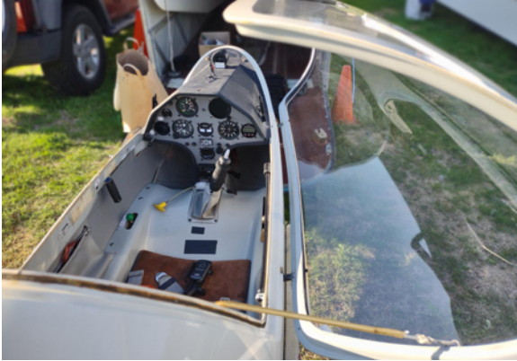
Terry Crippen of PSSA, is the proud new owner of this Discus B. He added an LXNAV S100 Vario Flight Computer with Flarm Fusion and an Oudie N.
