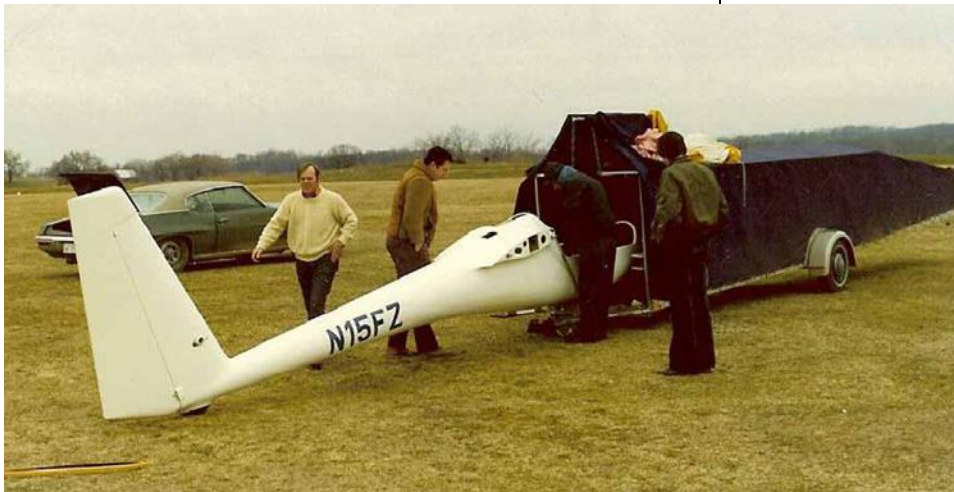
Preparing to rig Foxtrot Zulu. We built the trailer from plans given to us by Schleicher – and it was very klugey. The fuselage rolls in and out of the trailer on a wheeled dolly in two parallel tracks. The wings are in slings, suspended from the tube ceiling on either side of the fuselage. It was a recipe for trailer rash.
