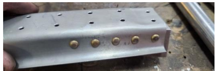
New engine mount stringer prior to installation
