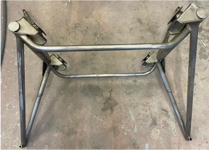
Engine mount, stripped, inspected and ready for paint
