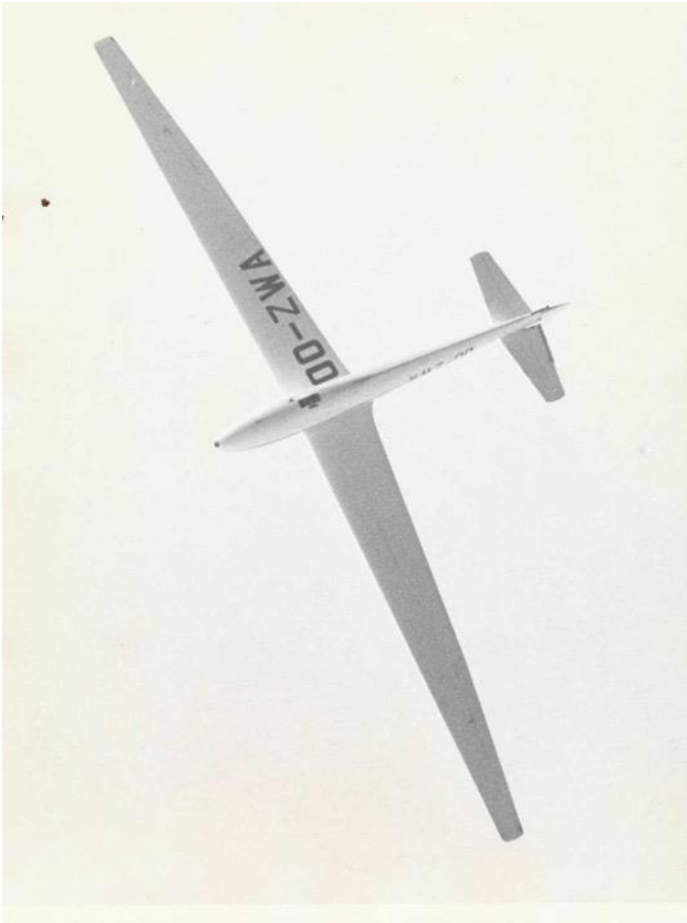
The S.H.A.P.E. Gliding Club's best Ka-6CR sailplane, Whiskey Alpha, directly overhead in this low-level aerial photo. OO is the international country designation for a Belgian-registered aircraft (as "N" is the designation for United States-registered aircraft). The Ka-6CR has a 15m wing span and fixed main landing gear. Performance is a modest 34:1.
