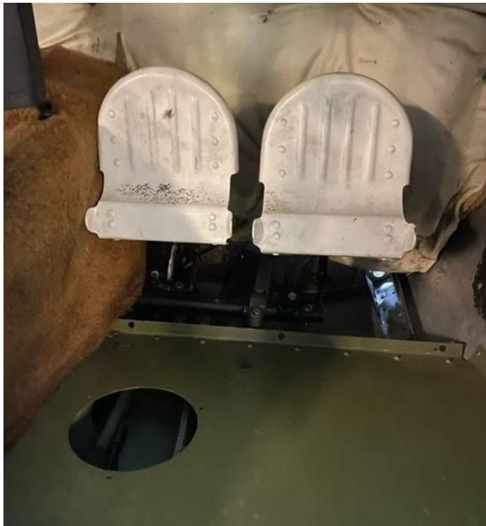
Left side with rudder pedal assembly back together after stringer repair
