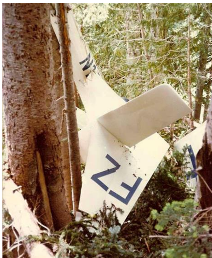
It's difficult to figure out the juxtaposition of Foxtrot Zulu's vertical tail and fuselage in this photo. Aft of the N-number on the fuselage, you can see the jagged break in the tail cone in front of the rudder and elevator. The tail section snapped off on impact and fell crashing downward, landing upside down but was hung up by the control cables to the tail surfaces. Otherwise, the tail was fairly intact. The cockpit radio's antenna is located in the tail, and the co-axial cable to the antenna was broken. I didn't have the presence of mind to even try the radio, as the instruments were a mess, and I figured they were all toasted.
